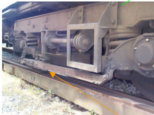
Mk.6 Motor Bogie (leading) showing PNS8 design shoe gear Class 411/6 & 412
