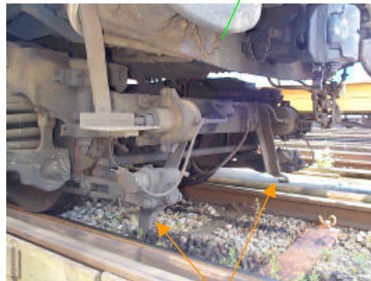
Mk.6 Motor Bogie (leading) showing guard irons Class 411/6 & 412
