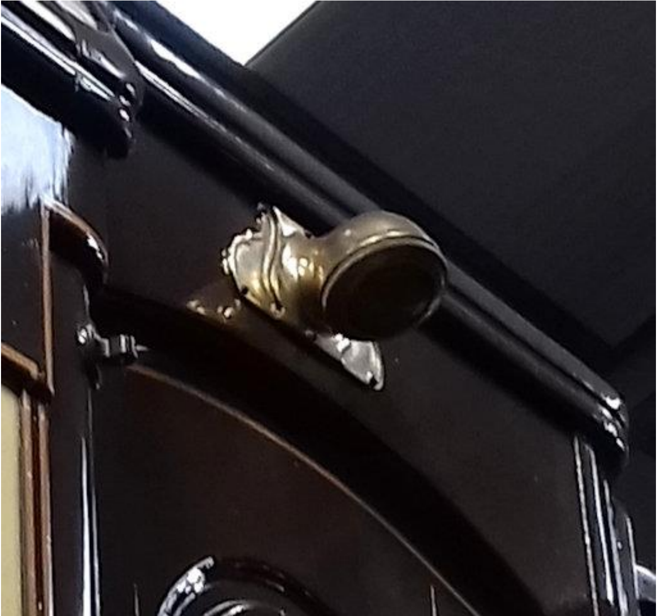
Embarkation light as fitted on CAR No. 54.
