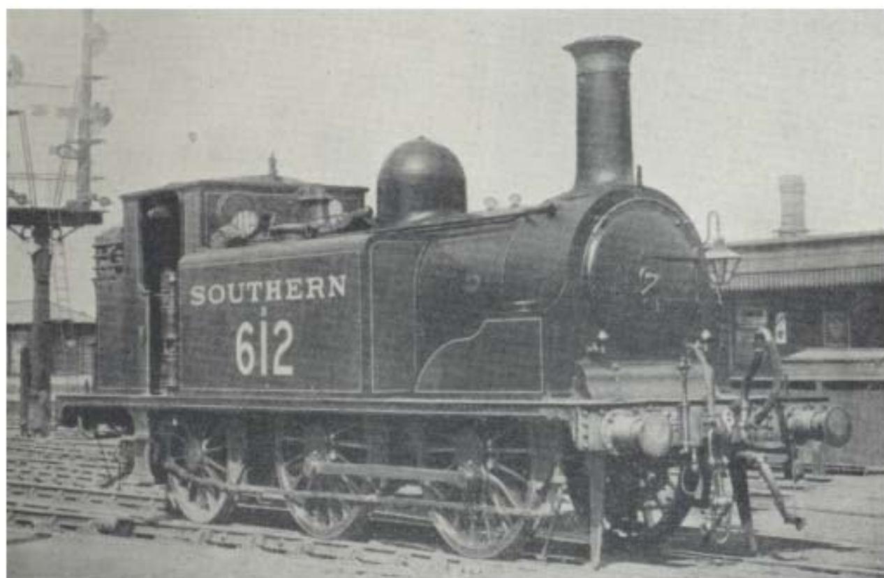
Photo] One of the last "D1s" to retain the copper-capped chimney, No. B612 at New Cross in 1926 [O. J. Morris
