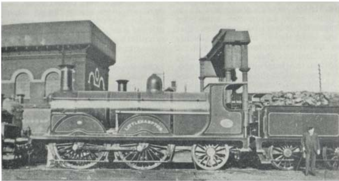
One of Stroudley's 0-4-2s, No. 172, "Littlehampton," in the locomotive yard at Brighton about 1904. The lifting gantry is in the background
