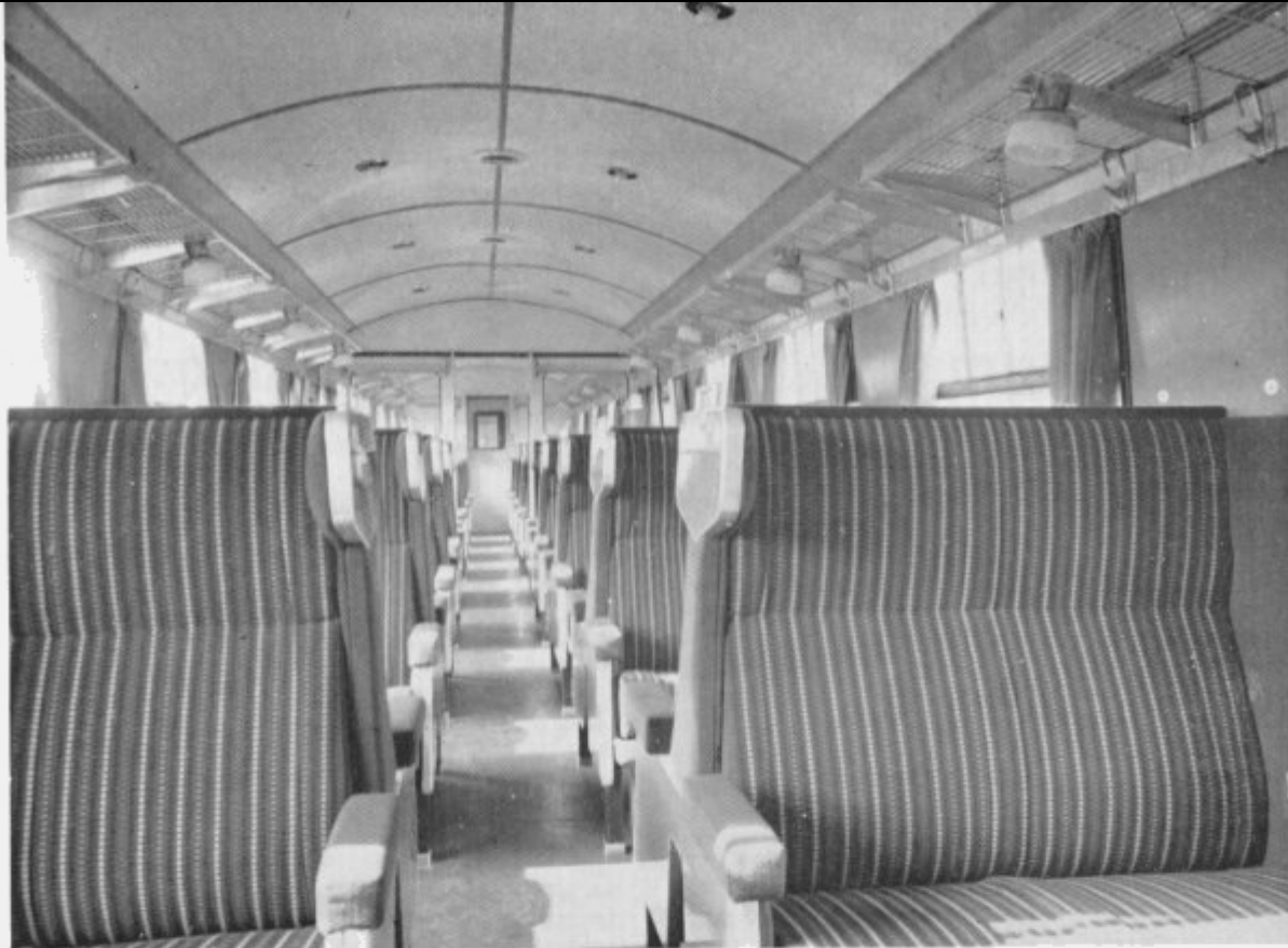
Interior of second-class trailer, which seats 72 passengers. Luggage-rack lights replace the usual shoulder lamp fittings
